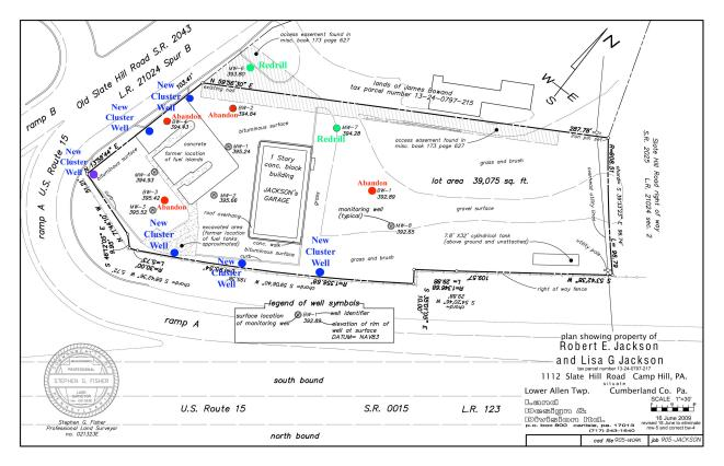
All wells and soil borings shall be completed consistent with consistent with the guidelines established within PaDEP's December 2001 Groundwater Monitoring Guidance Manual, a copy of which is included in Attachment 1. Bidders shall identify construction details of all proposed wells and borings.
