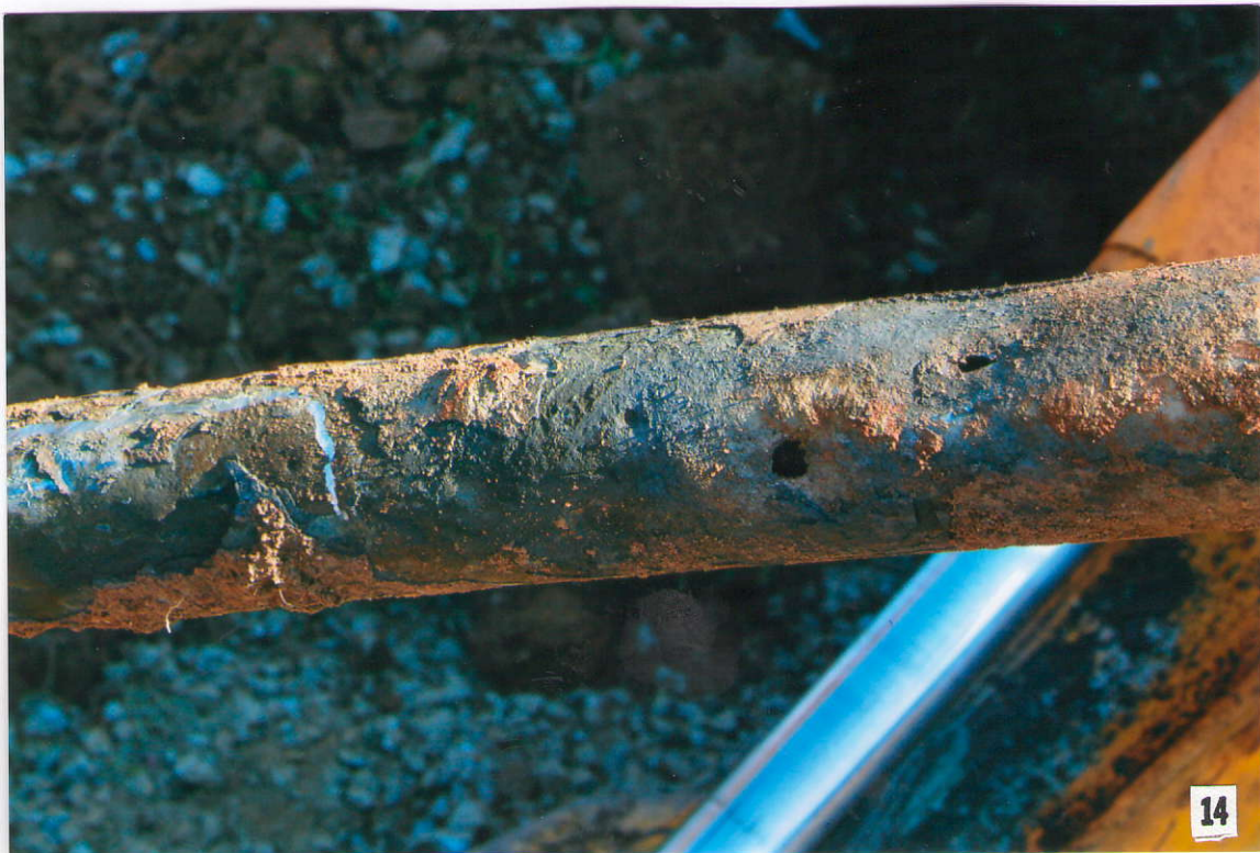
Photograph #10 – Holes in supply line from Tank #004
